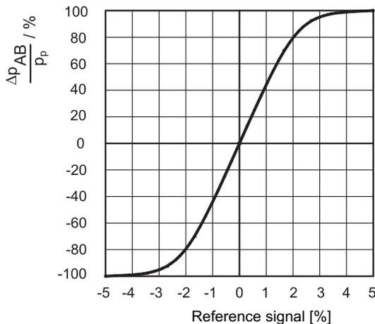
The diagram on the left shows the valve pressure gain, expressed as % of the ratio between the port pressure variation in A or B ( $\Delta p_{AB}$ ) and the P system pressure, according to the reference signal. Practically, the pressure gain states the valve reaction towards external disturbances aimed at changing the actuator position.
